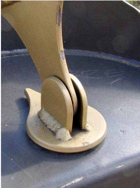
Figure J-18. Paint on viewing tubes and housings is chipped, scratched, and scraped.
